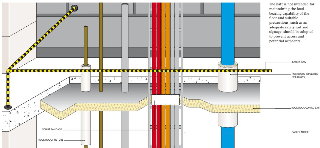
The Batt is not intended for maintaining the load-bearing capability of the floor and suitable precautions, such as an adequate safety rail and signage, should be adopted to prevent access and potential accidents.
